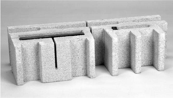
Figure 6.9 A CMU (concrete masonry unit) which uses two slotted Helmholtz absorbers to provide bass absorption, DiffusorBlox<sup>®</sup> (one slot is difficult to see).
