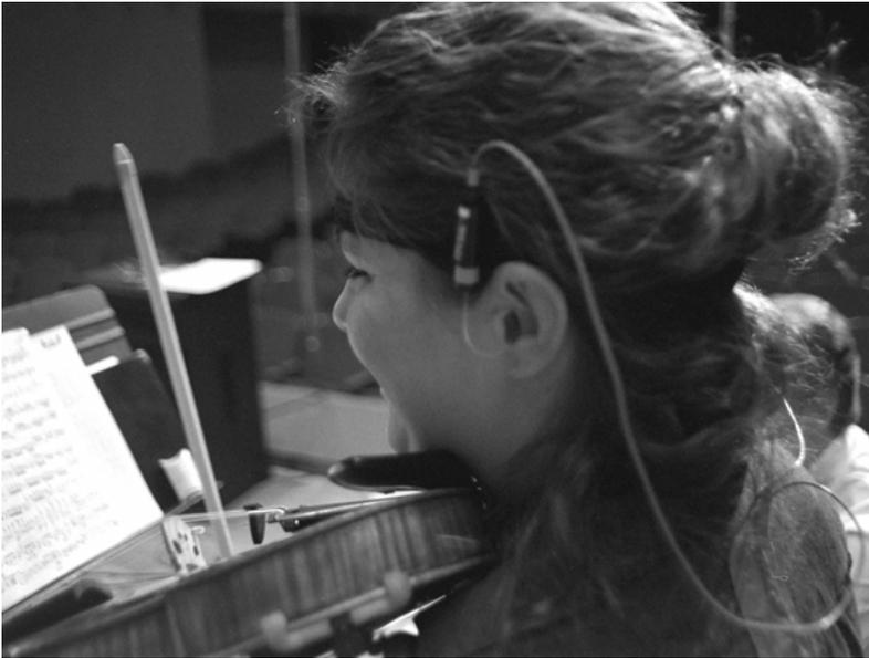
*Figure 2.27* In the ear probe microphone inserted into the ear canal of the 1st violinist. Microphone is inserted to a point just in front of the ear drum (after D'Antonio [22]).
