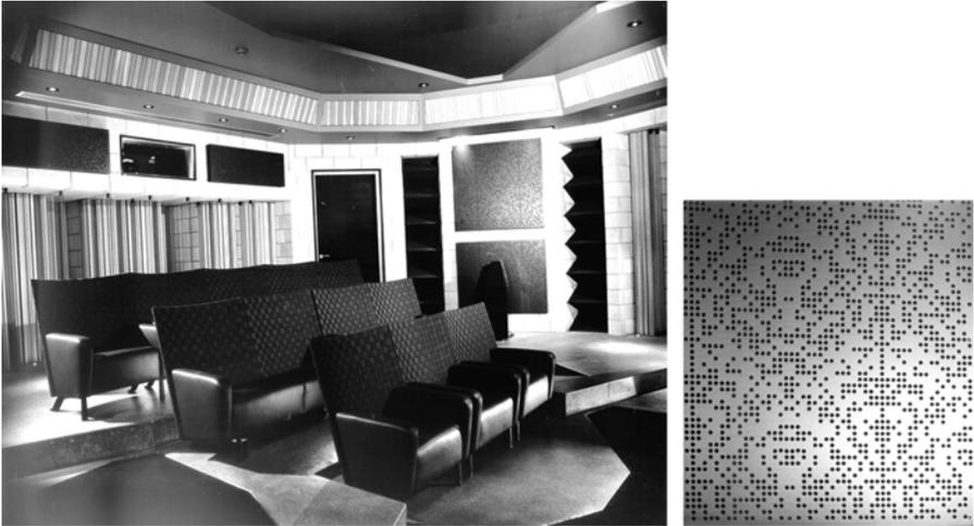
*Figure 11.3* Example application of planar hybrid surface (BAD panel) in a home theatre (left). The BAD panels are to the left of the seating and are also shown magnified in the right picture.
