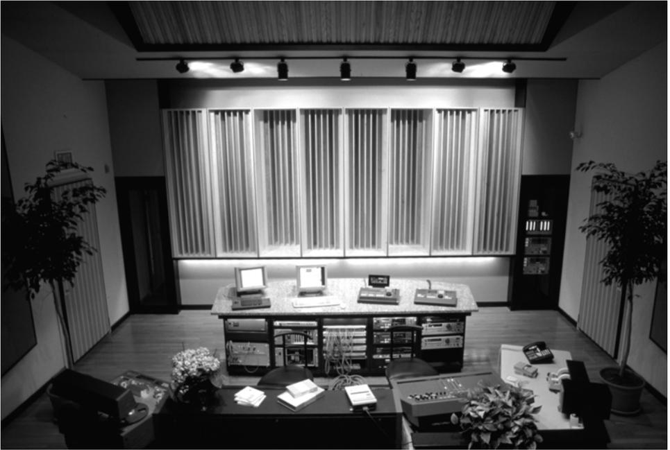
*Figure 2.12* Gateway Mastering, Portland, ME showing a fractal diffusing rear wall Diffraactal<sup>®</sup> (photo courtesy of Gateway Mastering + DVD).
