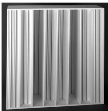
Figure 9.26 A Difractal<sup>®</sup>, which imbeds high frequency diffusers within a low frequency diffuser to deal with periodicity, absorption and bandwidth problems (top figure after D'Antonio and Konnert [7]).
