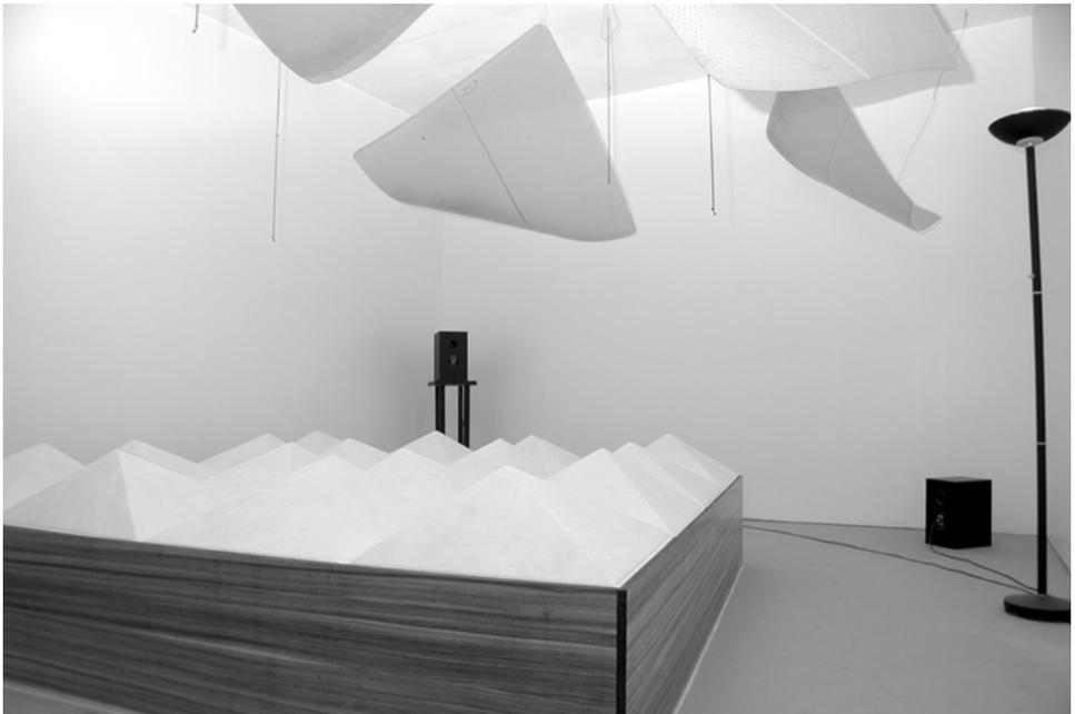
*Figure 2.19* A small reverberation chamber (photo courtesy of RPG Diffusor Systems Inc.).
