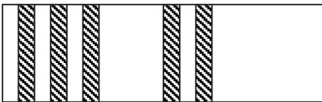
Figure 11.6 A 1D hybrid surface. The cross-hatched patches are absorptive and the clear patches reflective (or vice versa).
