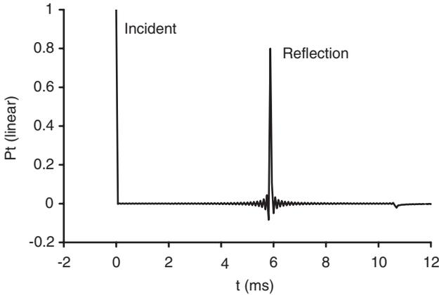
Figure 10.3 Time response for incident and scattered sound from a plane surface (not the same case as Figure 10.2).
