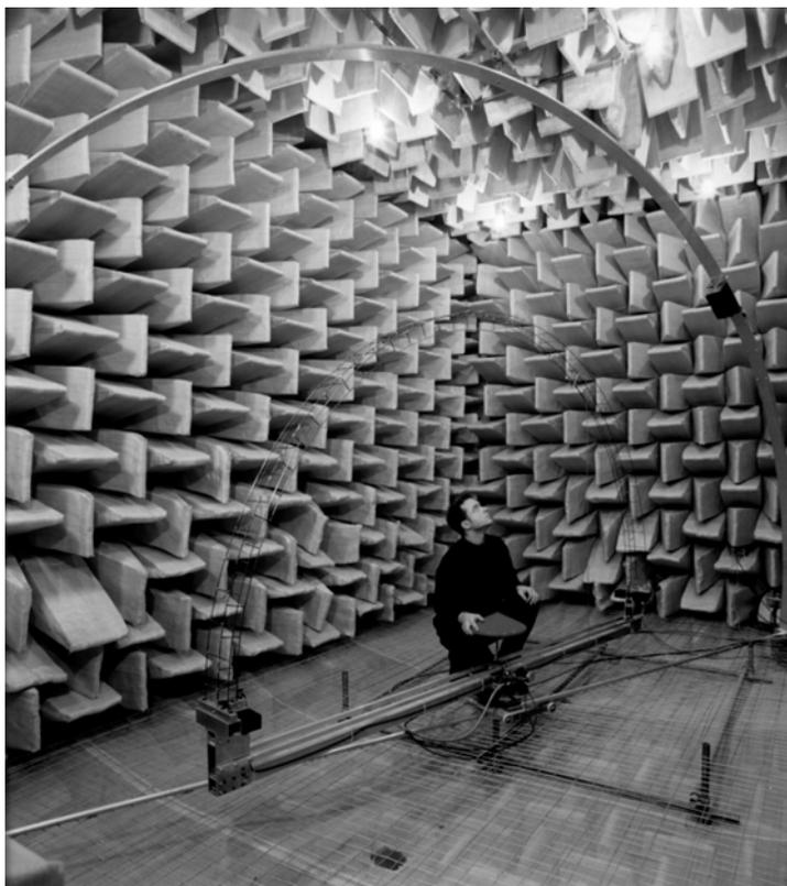
*Figure 4.3* A system for measuring the scattering from a surface over a hemisphere. The diffuser being tested is the small pyramid in the centre. The source arc is most obvious, the receiver arc is acoustically transparent and so is difficult to see (after AES [6], photo courtesy of University of Salford).
